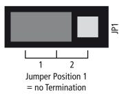
If you want to switch-off the termination, remove carefully the jumper from the two pins of position 2 of the socket and plug it onto the two pins of position 1 (see adjacent sketch).
