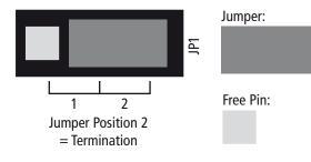
When the MC-3+USB is shipped, the BNC-based Word Clock input connector is terminated internally with 75  $\Omega$ . Therefore, one jumper is put on two pins - Position 2 - of the 3-pin socket JP1. (see adjacent sketch on page 25).
